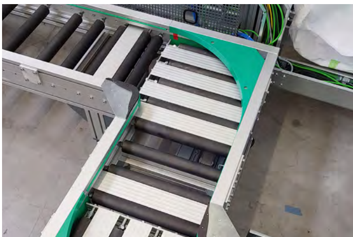
The Delta deflection system of the RMS enables uninterrupted transport around curves.
