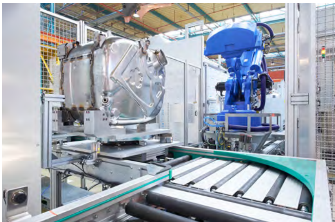
The RMS workpiece carrier transfer system was designed for heavy-duty transport.
