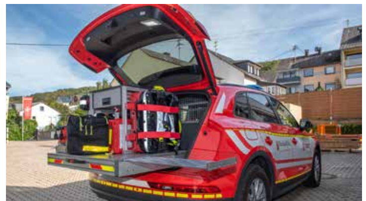
Interior fit outs with telescopic equipment racks can also be implemented quickly and easily for cars.
